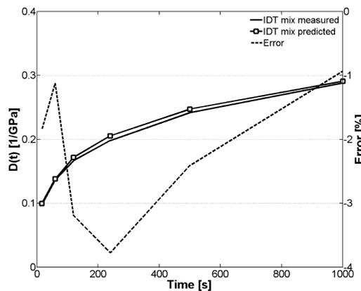
Fig. 6. Representative Creep Curves for Case A.
