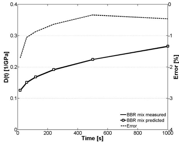
Fig. 7. Representative Creep Curves for Case B.
