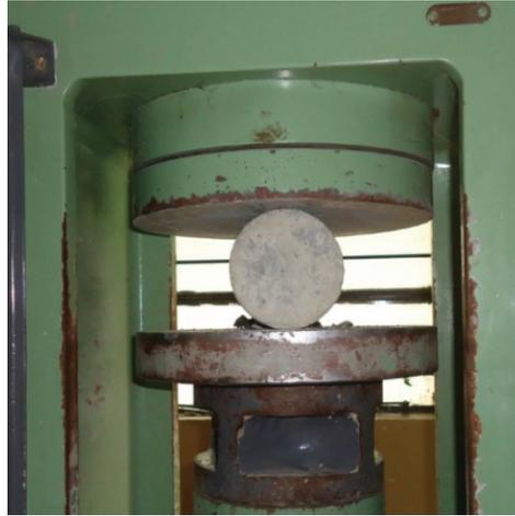
Fig. 7. Split tensile testing set up
