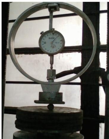
Fig. 3. CBR testing machine
