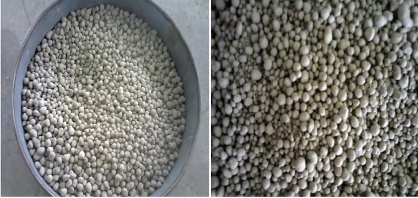
Fig. 2. Fly ash lightweight aggregate
