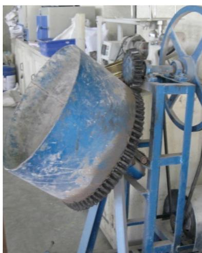
Fig. 1. Disc pelletizer machine
