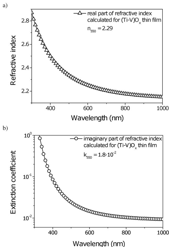
Fig. 6. Real (a) and imaginary (b) parts of refractive index calculated for (Ti-V)O<sub>x</sub> thin film
