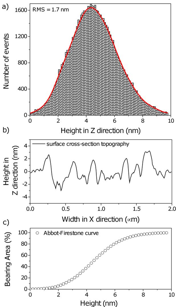
Fig. 3. Analysis results of AFM investigations: a) height distribution of grains size in Z direction, b) surface cross-section topography and c) Abbott-Firestone curve of (Ti-V)O<sub>x</sub> thin film
