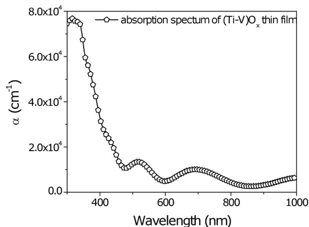
Fig. 7. Absorption spectrum of (Ti-V)O<sub>x</sub> thin film
