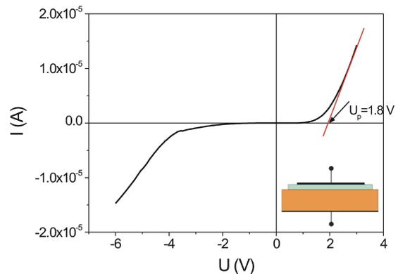
Fig. 10. I-V characteristics of TOS-Si heterojunction based on (Ti-V)O<sub>x</sub> thin film measured in the lateral configuration.  $U_p$  – threshold voltage
