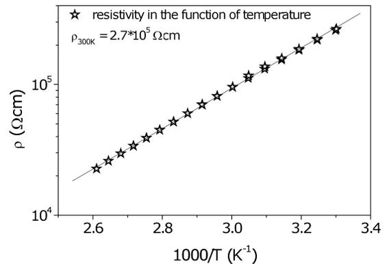
Fig. 9. Resistivity in the function of temperature of (Ti-V)O<sub>x</sub> thin film deposited on Corning glass substrates
