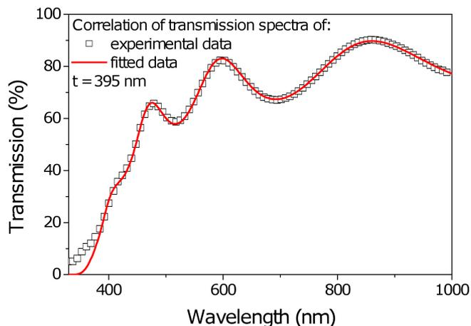
Fig. 5. Correlation of transmission spectra of (Ti-V)O<sub>x</sub> thin film determined experimentally and by reverse engineering method. Designation: *t* – thickness of the thin film
