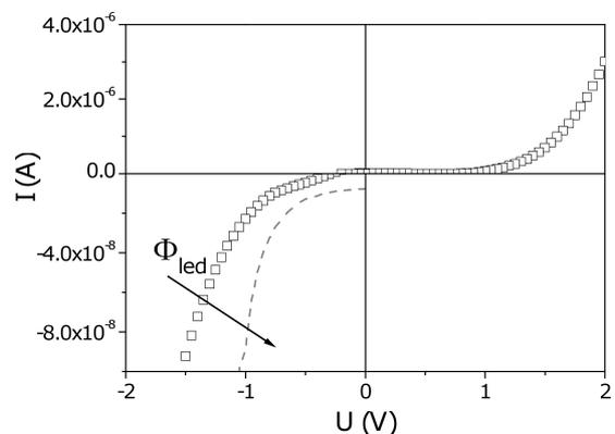
Fig. 11. Influence of light illumination on I-V characteristics of TOS-Si heterojunction based on (Ti-V)O<sub>x</sub> thin film measured in the lateral configuration
