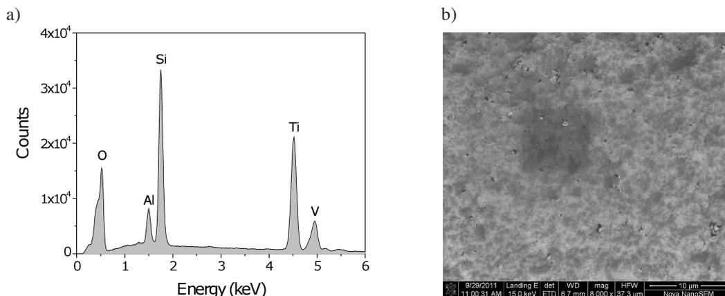
Fig. 1. Images of: a) EDS spectrum and b) surface of (Ti-V) $O_x$  thin film performed by SEM measurements
