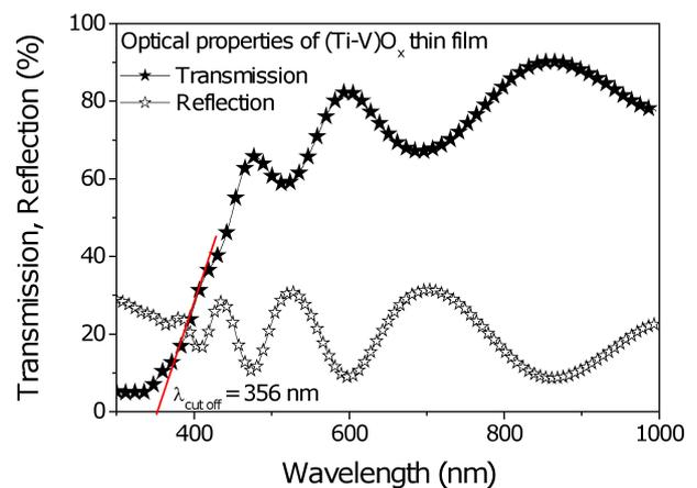
Fig. 4. Transmission and reflection spectra of (Ti-V)O<sub>x</sub> thin film deposited on Corning glass substrate
