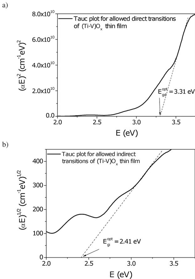
Fig. 8. Tauc plots for allowed: a) direct and b) indirect transitions of (Ti-V)O<sub>x</sub> thin film. Designations:  $E_{gd}^{opt}$  – optical band gap for direct transitions,  $E_{gi}^{opt}$  – optical band gap for indirect transitions
