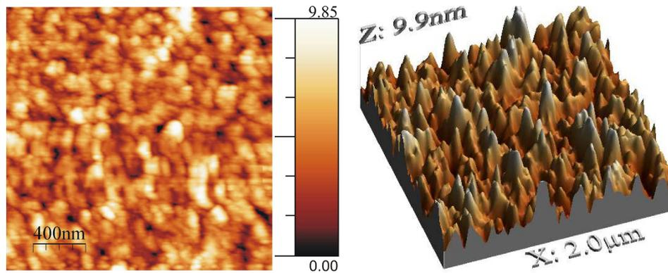
Fig. 2. AFM images of the surface topography of (Ti-V)O<sub>x</sub> thin film
