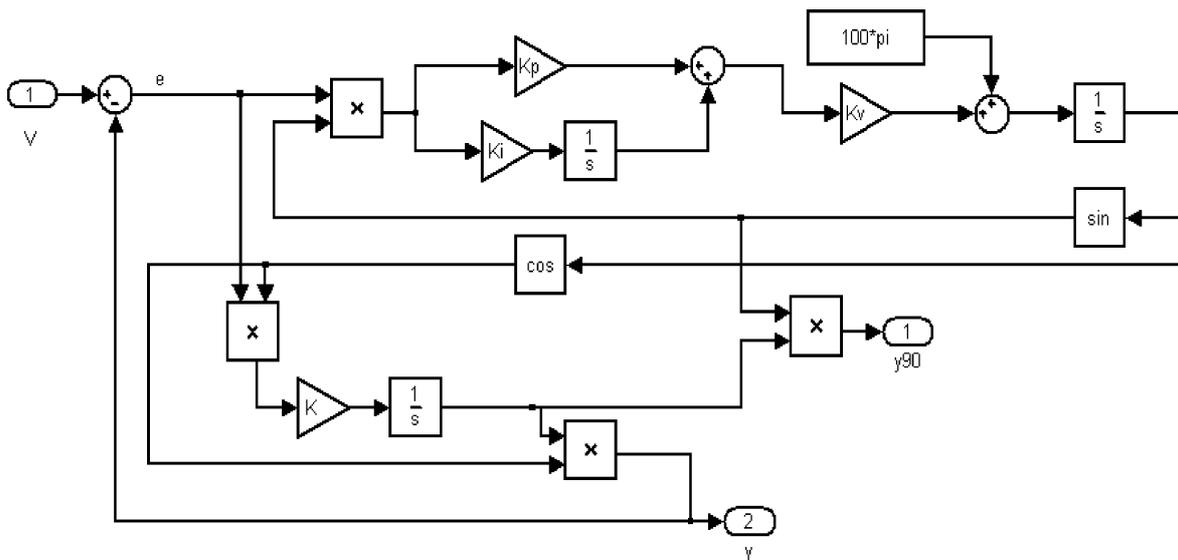
Fig. 4. Diagram of EPLL
