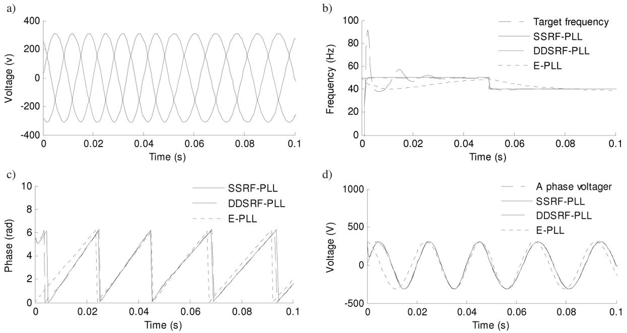
Fig. 8. Frequency and phase and voltage locked of three PLL technologies at frequency deviation
