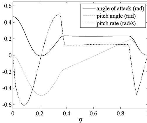
Figure 11. Time optimal states versus non-dimensional time.
