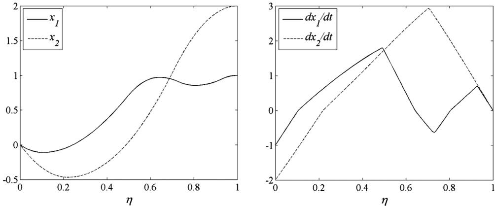
Figure 9. Time optimal states versus non-dimensional time.
