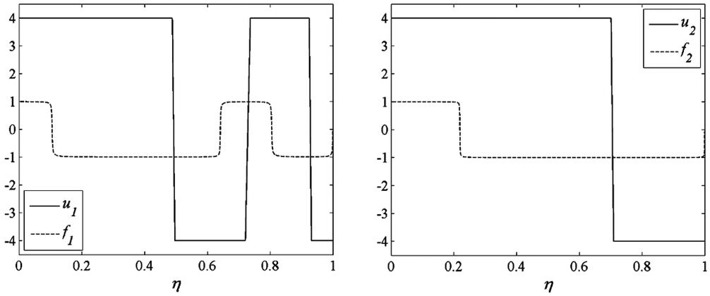
Figure 10. Time optimal controls and frictional forces versus non-dimensional time.
