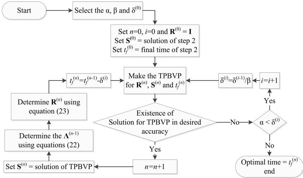
Figure 1. Flowchart of minimum time calculation (last phase).
