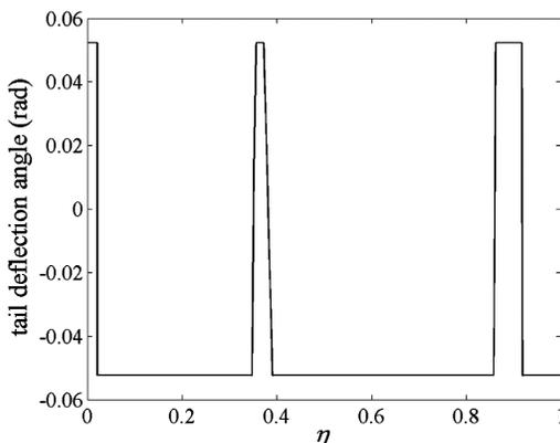
Figure 12. Time optimal control versus non-dimensional time.
