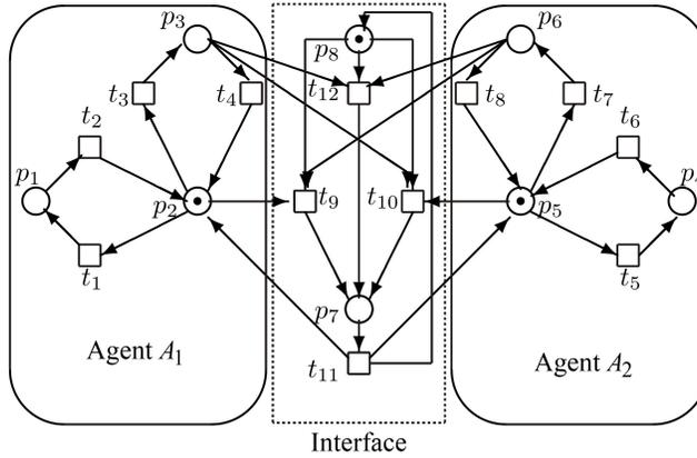
Figure 6. The P/T PN model of the negotiation process.
