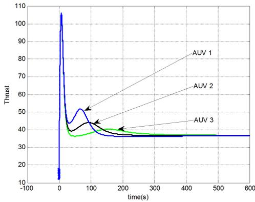
Figure 22: Thrust of three AUVs for circular path using SMC.
