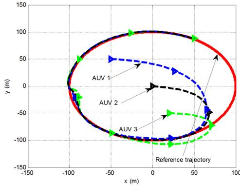
Figure 16: Formation of circular path of three AUVs following virtual leader using adaptive SMC.
