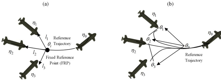
Figure 7: Formation path following virtual leader using (a) Passivity Controller (b) SMC.
