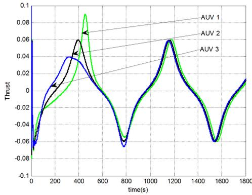
Figure 28: Thrust of three AUVs for sinusoidal path using SMC.
