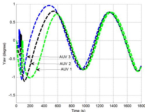
Figure 26: Euler angle of three AUVs for sinusoidal path using SMC.
