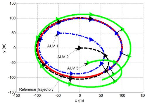
Figure 8: Formation of circular path of three AUVs following virtual leader using Passivity Controller.
