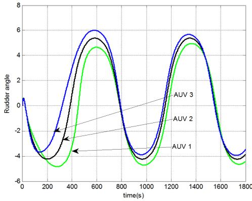
Figure 27: Rudder angle of three AUVs for sinusoidal path using SMC.
