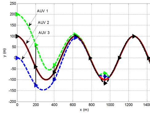
Figure 19: Tracking error of three AUVs following virtual leader using adaptive SMC for sinusoidal path.
