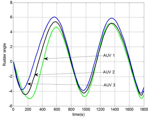
Figure 30: Rudder angle of three AUVs for sinusoidal path using adaptive SMC.
