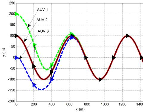
Figure 14: Formation of sinusoidal path of three AUVs following virtual leader using SMC for sinusoidal path.
