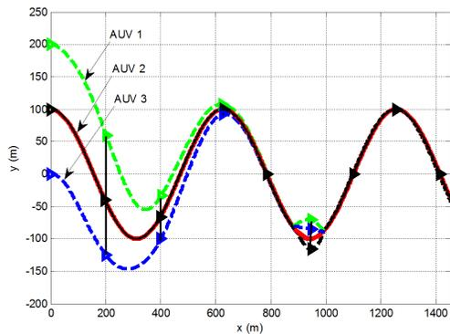
Figure 18: Formation of sinusoidal path of three AUVs following virtual leader using adaptive SMC.
