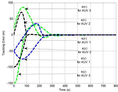
Figure 13: Tracking error of three AUVs following virtual leader using SMC for circular path.
