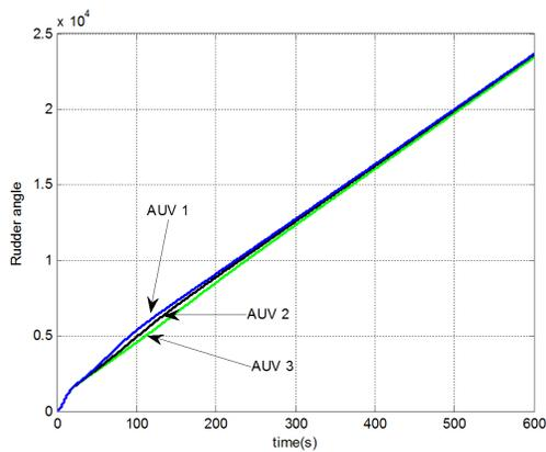
Figure 24: Rudder angle of three AUVs for circular path using adaptive SMC.
