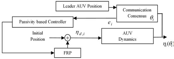
Figure 3: Formation control using passivity based controller.
