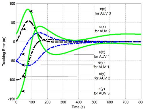
Figure 9: Tracking error of three AUVs following virtual leader using Passivity Controller for circular path.
