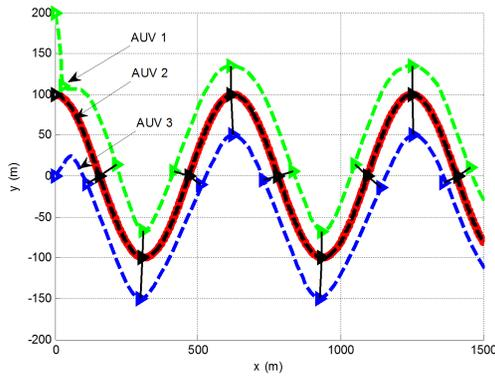
Figure 10: Formation of sinusoidal path of three AUVs following virtual leader using Passivity Controller.
