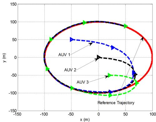
Figure 12: Formation of circular path of three AUVs following virtual leader using SMC.
