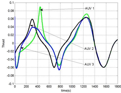
Figure 31: Thrust of three AUVs for sinusoidal path using adaptive SMC.
