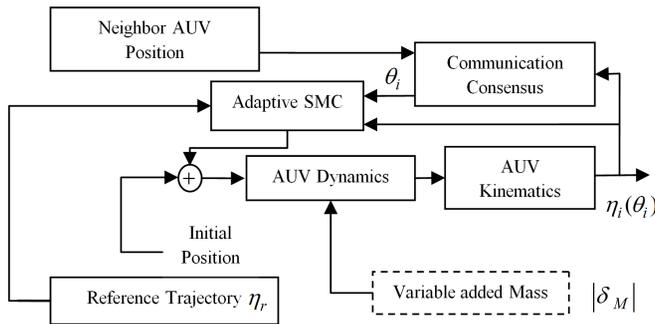
Figure 5: Formation control using adaptive SMC based controller with variable added mass.
