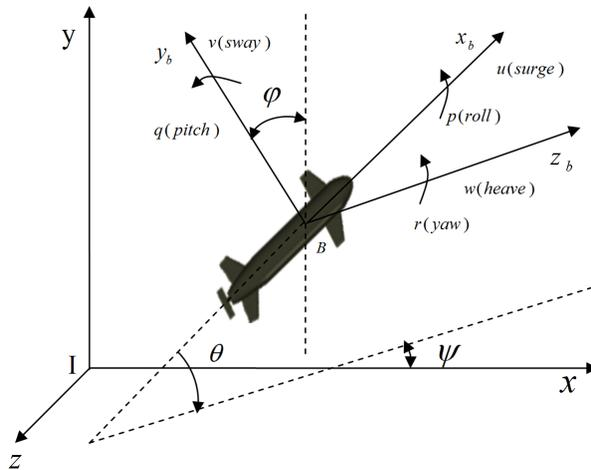
Figure 1: Inertial and body fixed frames of an AUV model.
