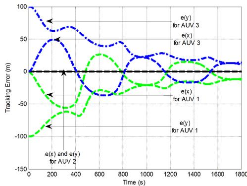
Figure 11: Tracking error of three AUVs following virtual leader using Passivity Controller for sinusoidal path.
