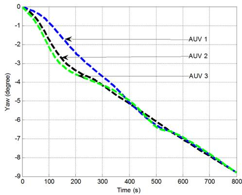
Figure 23: Euler angle of three AUVs for circular path using adaptive SMC.
