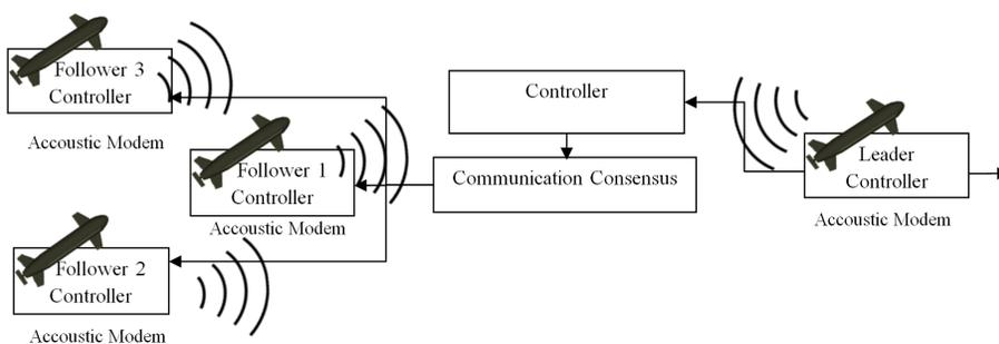
Figure 2: Formation Control of multiple AUVs using communication constraints.
