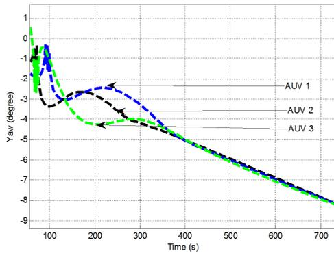
Figure 20: Euler angle of three AUVs for circular path using SMC.
