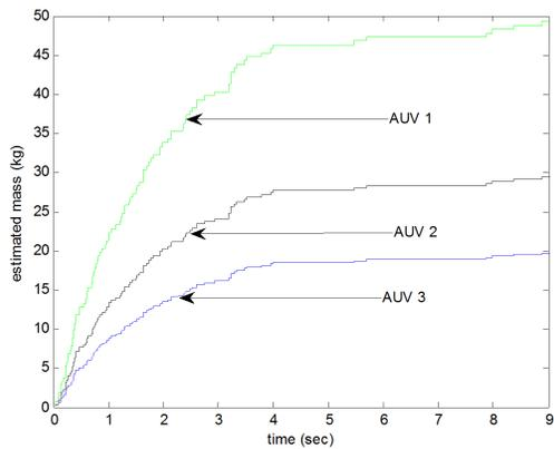
Figure 32: Estimated variable added mass for sinusoidal path using adaptive SMC.
