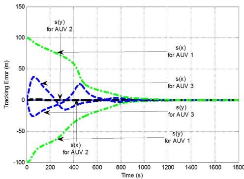
Figure 15: Tracking error of three AUVs following virtual leader using SMC.
