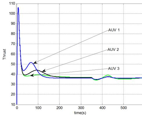
Figure 25: Thrust of three AUVs for circular path using adaptive SMC.
