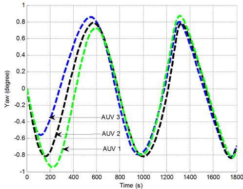
Figure 29: Euler angle of three AUVs for sinusoidal path using adaptive SMC.
