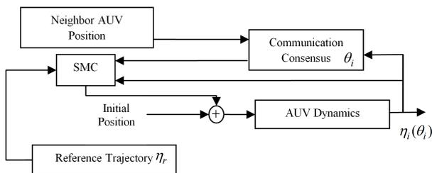
Figure 4: Formation control using SMC based controller.
