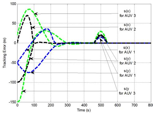
Figure 17: Tracking error of three AUVs following virtual leader using adaptive SMC for circular path.
