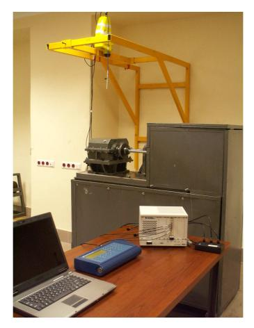
Fig. 2. Test stand FZG with measurement/recording equipment
