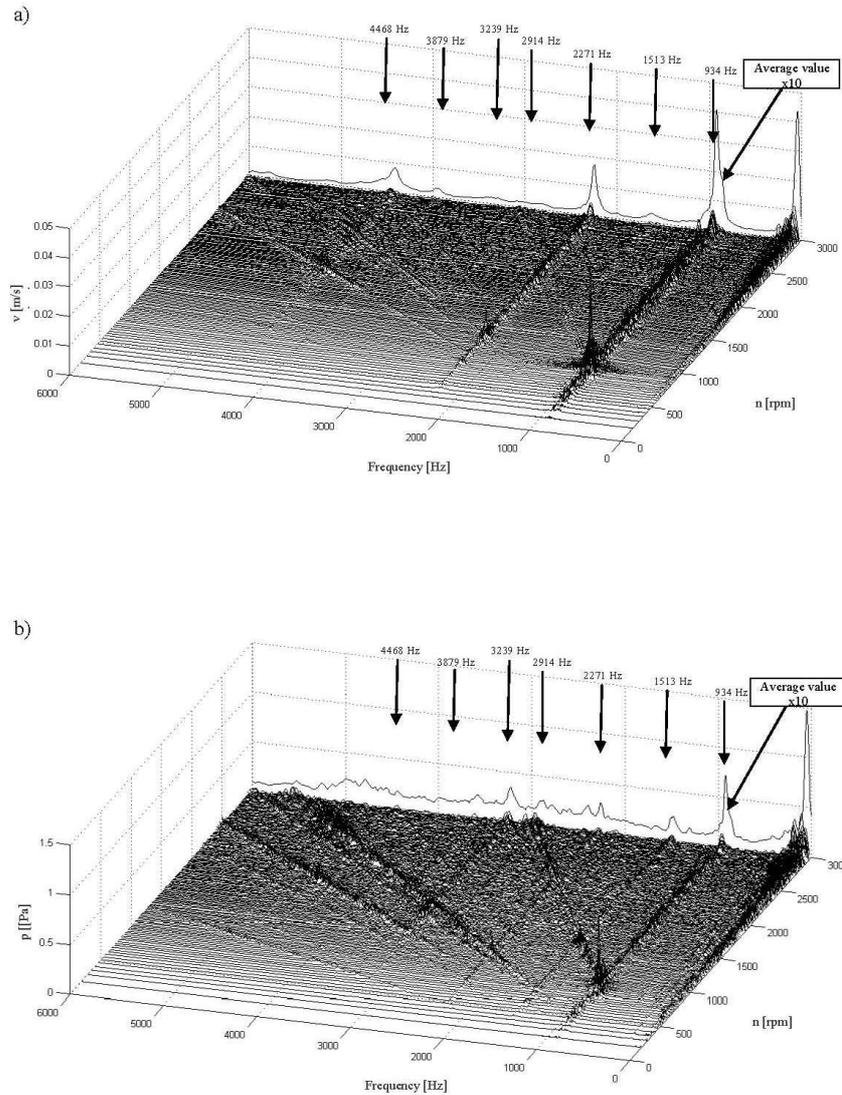
Fig. 5. Time-frequency distributions (pair 4): a) vibration velocities (K7),
