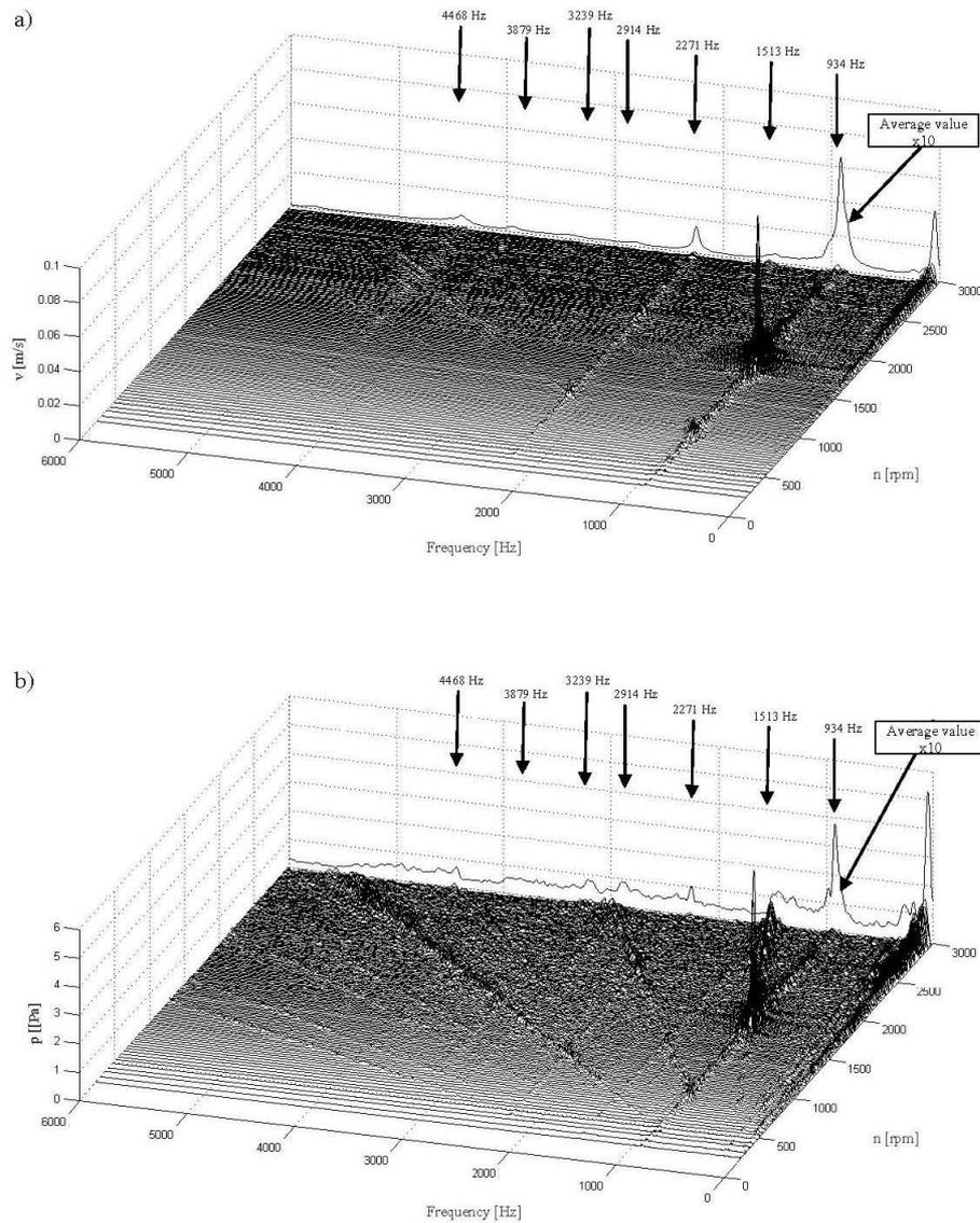
Fig. 4. Time-frequency distributions (pair 1): a) vibration velocities (K7),
