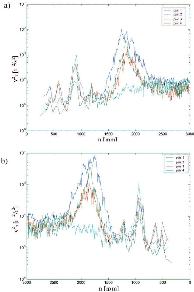
Fig. 6. The values of gearbox housing vibroactivity measure  $v_7^2$  in function of wheel shaft rotational speed: a) run up, b) run down
