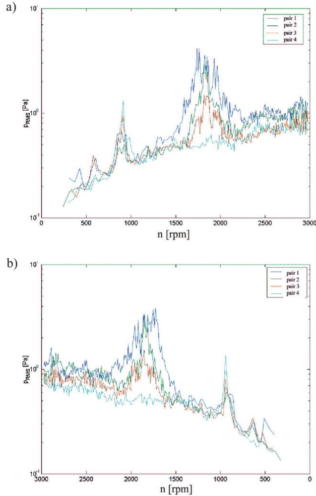
Fig. 7. Acoustic pressure in function of wheel shaft rotational speed: a) run up, b) run down
