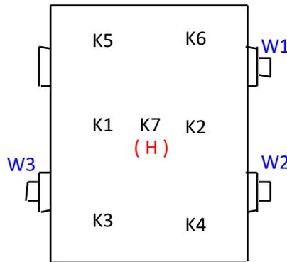
Fig. 3. Upper plate of the gearbox housing with marked vibration velocity measurement points K1-K7, as well as noise measurement point H
