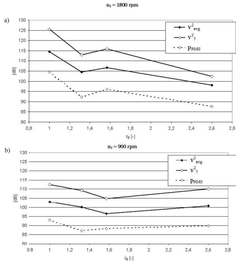
Fig. 8. Values of vibroactivity measure  $v_{avg}^2$ ,  $v_7^2$  and acoustic pressure  $p_{RMS}$  of gearbox housing in dependence on face contact ratio a) rotational speed  $n_2 = 1800$  rpm, b) rotational speed  $n_2 = 900$  rpm
