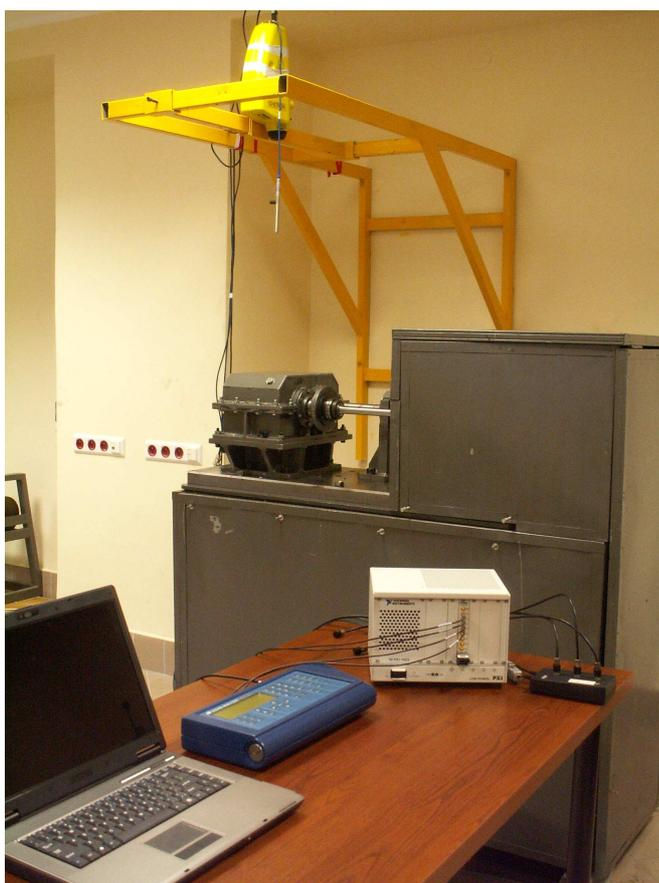
Fig. 2. Test stand FZG with measurement/recording equipment
