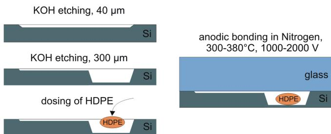
Fig. 3. Fabrication process in short
