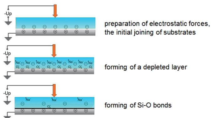
Fig. 1. Scheme of the chemical reaction steps in anodic bonding process of silicon and glass
