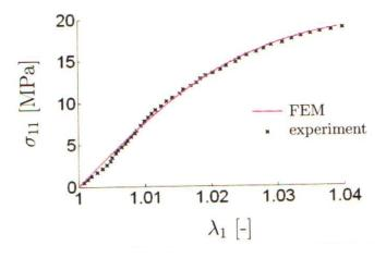
Fig. 5. Comparison of simple tension test data and FEM predictions
