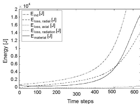
Fig. 10. Energy balance of the skull melting process
