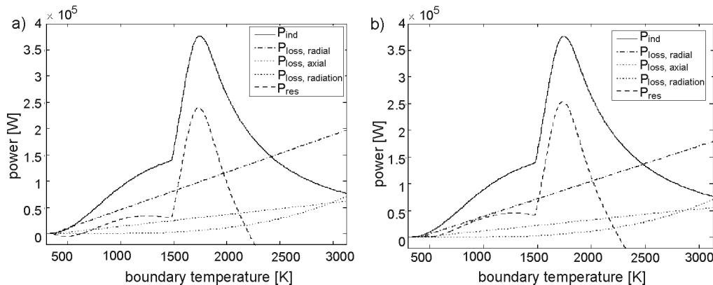
Fig. 9. Induced power, thermal losses and resulting power inside the target material:
