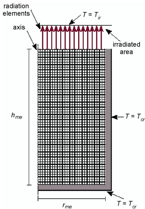
Fig. 7. Finite element model of the thermal computation
