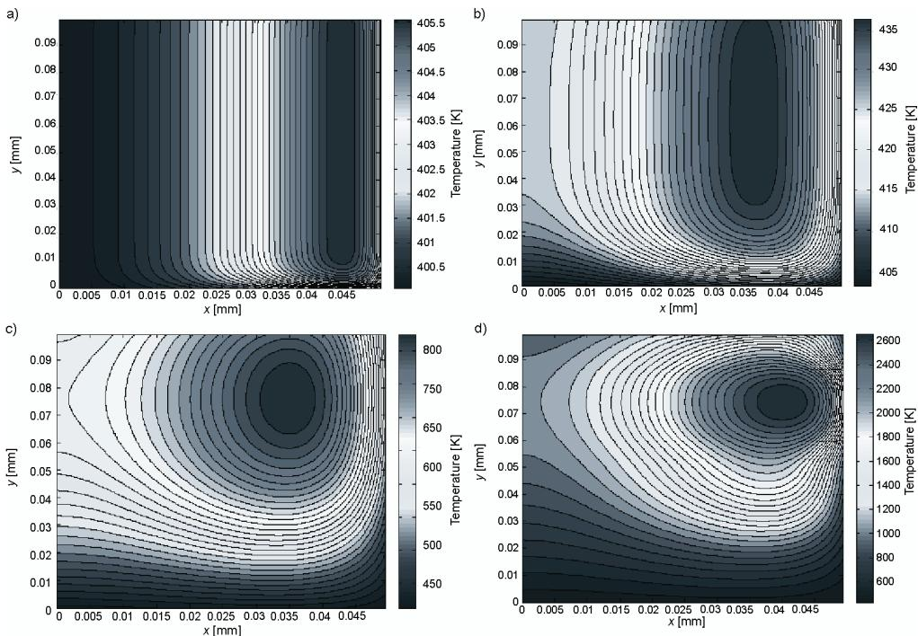
Fig. 11. Temperature distribution inside the target material at different time steps  $t$ :
