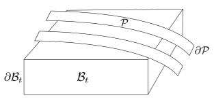
Fig. 1. A generic EMAT configuration.  $\mathcal{B}_t$  and  $\mathcal{P}$  are the regions occupied by the continuum material and a wire of the current-carrying coil, respectively. The corresponding boundaries are denoted by  $\partial \mathcal{B}_t$  and  $\partial \mathcal{P}$
