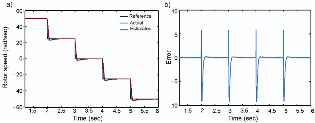
Fig. 4. Performance curves for test condition-1: (a) actual and estimated speed, (b) error between actual and estimated
