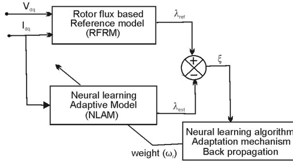
Fig. 1. Speed estimation using rotor flux based MRNLAS (RF-MRNLAS)
