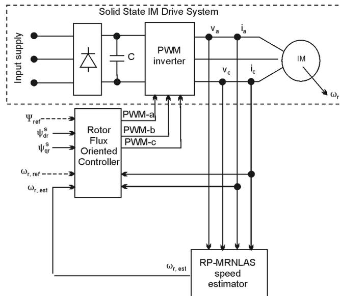
Fig. 3. Sensor-less indirect vector controlled IM drives with proposed RP-MRNLAS speed estimators
