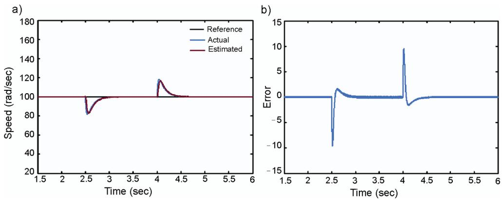
Fig. 5. Performance curves for test condition-2: (a) actual and estimated speed, (b) error between actual and estimated
