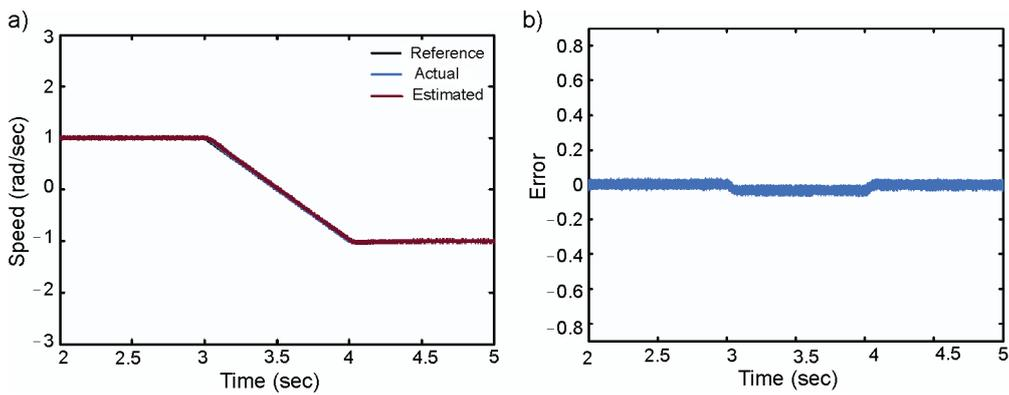
Fig. 8. Performance curves for test condition-5: (a) actual and estimated speed, (b) error between actual and estimated
