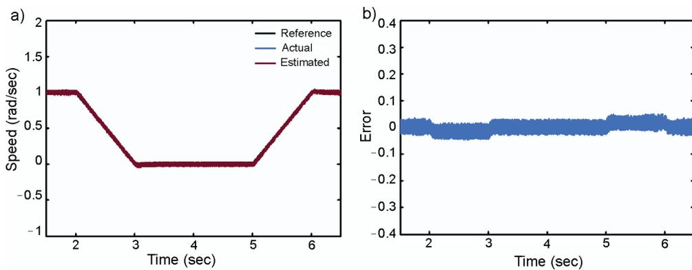
Fig. 9. Performance curves for test condition-6: (a) actual and estimated speed, (b) error between actual and estimated
