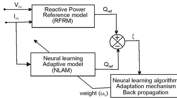
Fig. 2. Speed estimator using reactive power based MRNLAS (RP-MRNLAS)
