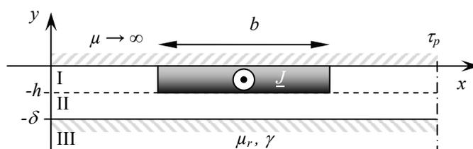
Fig. 1. Arrangement for analytical calculation of eddy current
