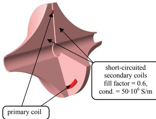
Fig. 12. Rotationally symmetric arrangement with high peak ratio  $I_2 / I_1$
