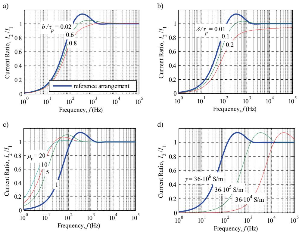
Fig. 2. Current ratio exceeding the value of one. The phenomenon occurs depending on parameters  $b/\tau_p$ ,  $\delta/\tau_p$ , and  $\mu_r$ , see a), b), c). A change of the conductivity  $\gamma$  shifts the frequency of the peak, see d)
