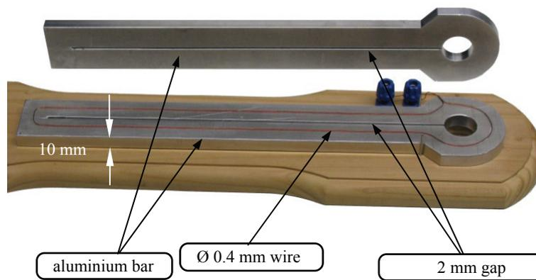
Fig. 5. Test assembly
