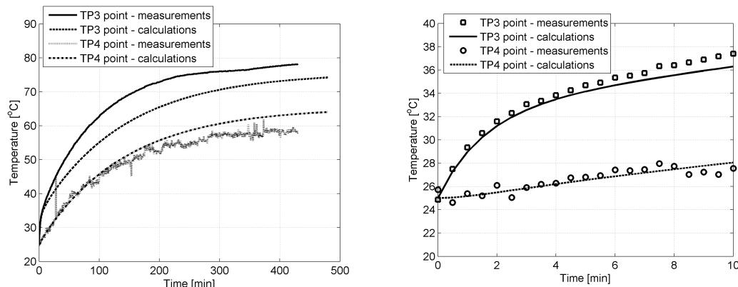
Fig. 8. Measurement verification ( $T_0 = 25^\circ\text{C}$ ,  $I = 1.2 \text{ A}$ ):
