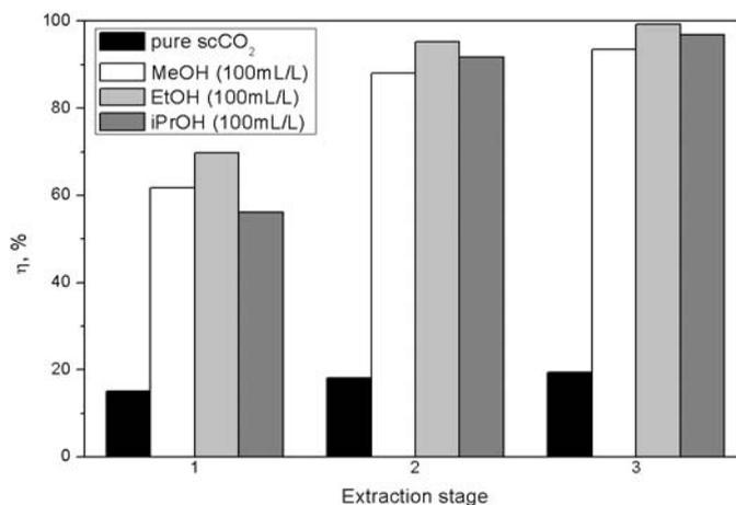
Fig. 6. Multi-stage extraction efficiency (70 °C, 18 MPa, 120 min, 100 mL/L organic solvent)
