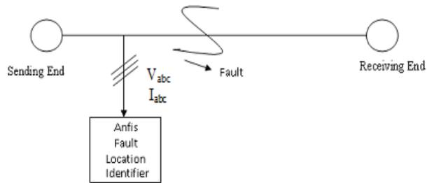
Fig. 2. Single line diagram of system model
