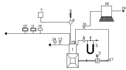
Fig. 2. Experimental set-up: 1 – engine, 2 – electical dynamometer, 3 – load box, 4 – orifice flow meter, 5 – U-tube water manometer, 6 – air box, 7 – fuel tank, 8 – pre-heater, 9 – burette, 10 – exhaust gas temperature indicator, 11 – AVL smoke meter, 12 – netel chromatograph NOx analyzer, 13 – outlet jacket water temperature indicator, 14 – outlet-jacket water flow meter, 15 – Piezo-electric pressure transducer, 16 – console, 17 – TDC encoder, 18 – Pentium Personal Computer, 19 – printer
