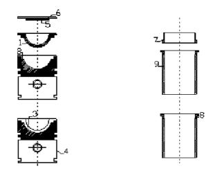
Insulated piston Insulated liner Ceramic coated cylinder head Fig. 1. Assembly details of air gap piston liner, air gap insulated liner and ceramic coated cylinder head: 1 – crown; 2 – gasket; 3 – air gap; 4 – body; 5 – ceramic coating; 6 – cylinder head; 7 – insert; 8 – air gap; 9 – liner
