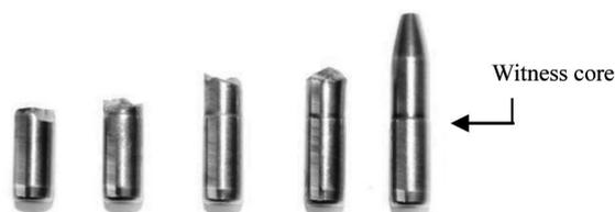
Fig. 5. 7.62 mm AP bullet core after shot tests
