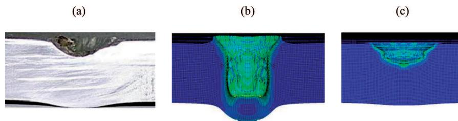
Fig. 13. Comparison between experimental and numerical penetration depth of 8 mm 30PM plates impacted by 7.62 AP bullet: (a) experiment result, (b) MJC strain hardening parameters determined from tensile tests; (c) MJC strain hardening parameters determined from compression tests
