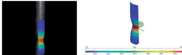
Fig. 2. True strain measurements during uniaxial tensile test using 3D deformation analysis
