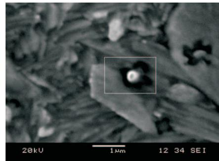
Fig. 7. SEM image of a spherical iron particle
