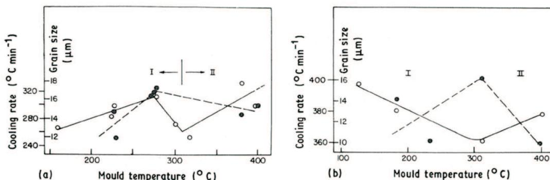
Fig. 8. The interdependence of the cooling rate ( $\bullet$ ) and  $\alpha$  grain size ( $\circ$ ) as a function of the pre-heating temperature of the die. (a) Graphite coating thickness 0.01 mm; (b) Graphite coating thickness 0.1 mm
