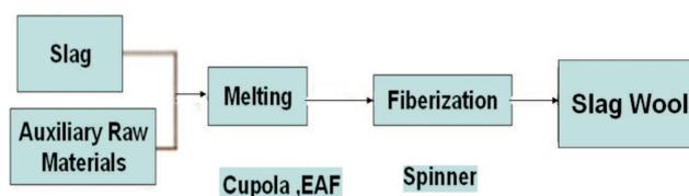
Fig. 1. Manufacturing process of BF slag wool [1]
