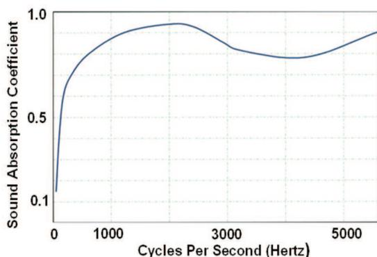
Fig. 2. Variation of frequencies with sound absorption coefficient of isolator
