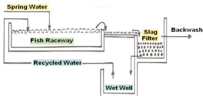
Fig. 6. Purifying trout farm water by BF slag
