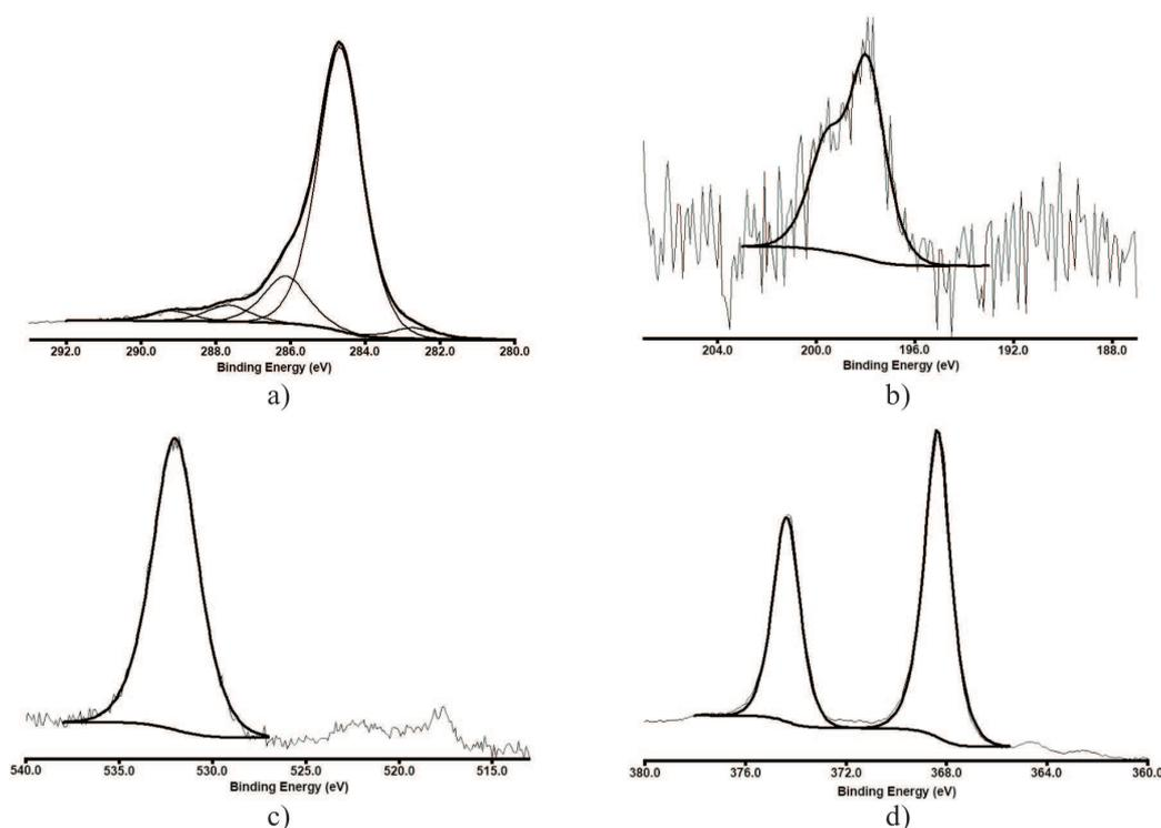
Fig. 6. XPS spectra of silver nanoparticles acquired in 0.001M LiClO<sub>4</sub> – C<sub>2</sub>H<sub>5</sub>OH solution, (E=1V), t=3h, T = 298 K in the bands: a) C 1s, b) Cl 2p, c) O 1s, d) Ag 3d
