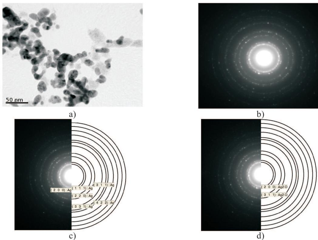
Fig. 4. TEM analysis of silver nanoparticles acquired during chronoamperometric polarization in alcoholic solutions of 0,001M  $\text{LiClO}_4$  ( $\text{C}_2\text{H}_5\text{OH}$ ,  $E=1\text{V}$ ,  $t=3\text{h}$ ,  $T=298\text{K}$ ): a) morphology, b) electron diffraction, c) cubic silver match, d)  $\text{Ag}_2\text{O}$  match
