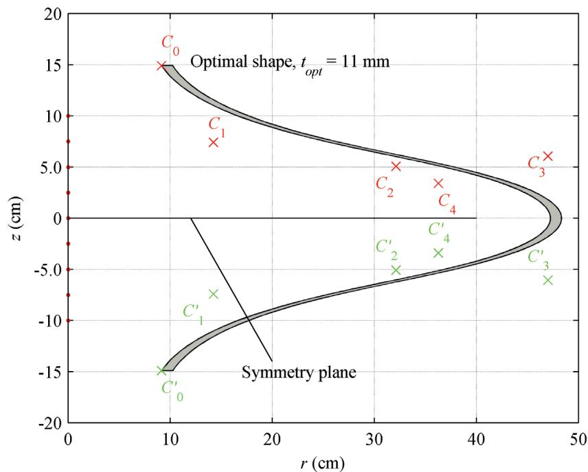
Fig. 6. Optimal shape of the solenoid for desired magnetic field  $H_0 = 45$  kA/m with determined  $t_{opt} = 11$  mm
