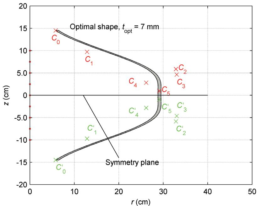
Fig. 4. Optimal shape of the solenoid for desired magnetic field  $H_0 = 35 \text{ kA/m}$  with determined  $t_{\text{opt}} = 7 \text{ mm}$
