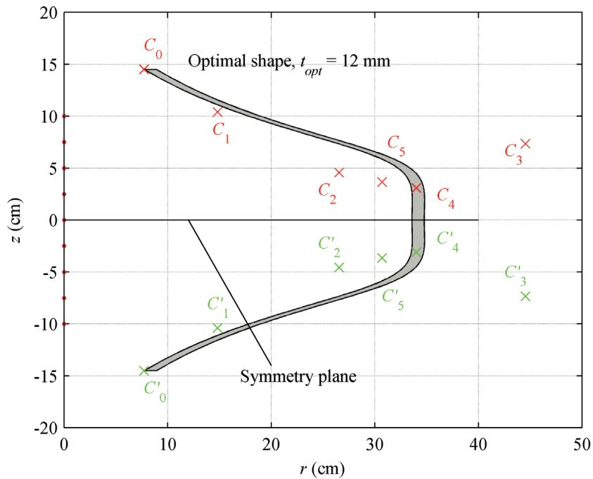
Fig. 8. Optimal shape of the solenoid for desired magnetic field  $H_0 = 55 \text{ kA/m}$  with determined  $t_{\text{opt}} = 12 \text{ mm}$
