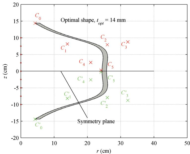
Fig. 10. Optimal shape of the solenoid for desired magnetic field  $H_0 = 75$  kA/m with determined  $t_{\text{opt}} = 14$  mm
