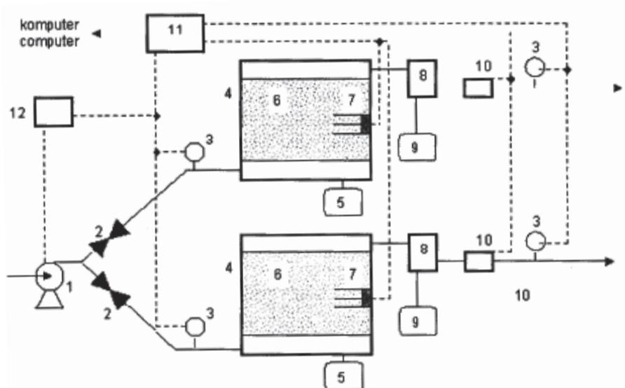
Fig. 1. Schematic diagram of the bioreactor: 1 – pump, 2 – flow regulator, 3 – flow meter, 4 – isolated chambers, 5 – drained liquid container, 6 – composted mass, 7 – sensors array, 8 – air cooling system, 9 – condensate container, 10 – multiplate gas sensor array, 11 – 32 channel recorder, 12 – 1lr pump steering system air
