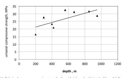
Fig. 14. Relation between compressive strength of semi-bright coal with interbedding of dull coal and deposition depth in the USCB (Bukowska 2012)
