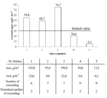
Fig. 2d. The average composition of treated sewage outflowing from wastewater treatment plants (total nitrogen) and limit values, 1 – Płoski, 2 – Ślubów, 3 – Irządze, 4 – Paszków, M – Mroczeń
