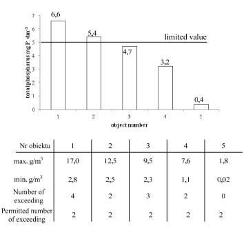
Fig. 2e. The average composition of treated sewage outflowing from wastewater treatment plants (total phosphorus) and limit values, 1 – Płoski, 2 – Ślubów, 3 – Irządze, 4 – Paszków, M – Mroczeń
