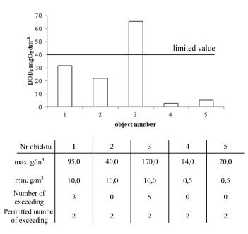
Fig. 2a. The average composition of treated sewage outflowing from wastewater treatment plants (BOD<sub>5</sub>) and limit values 1 – Płoski (hydroponic object), 2 – Ślubów (hydroponic object), 3 – Irządze (hydroponic object), 4 – Paszków (reed bed), 5 – Mroczeń (reed bed).
