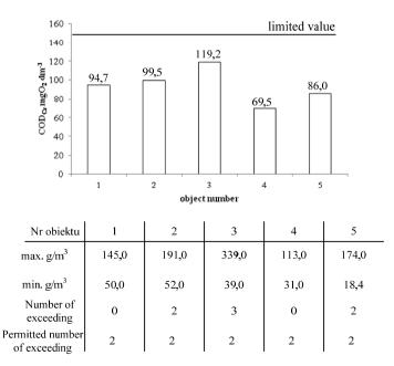
Fig. 2b. The average composition of treated sewage outflowing from wastewater treatment plants (COD) and limit values, 1 – Płoski, 2 – Ślubów, 3 – Irządze, 4 – Paszków, M – Mroczeń
