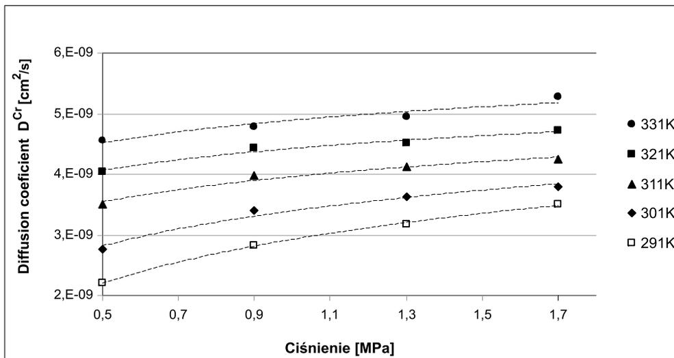
Fig. 4. The dependence of the diffusion coefficient on pressure
