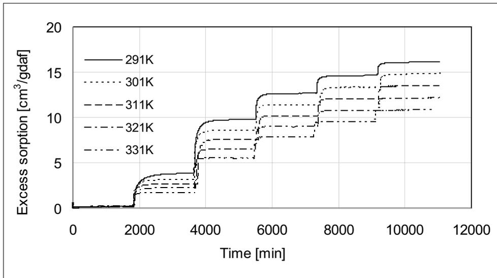
Fig. 5. Desorption kinetics of methane from coal at various temperatures
