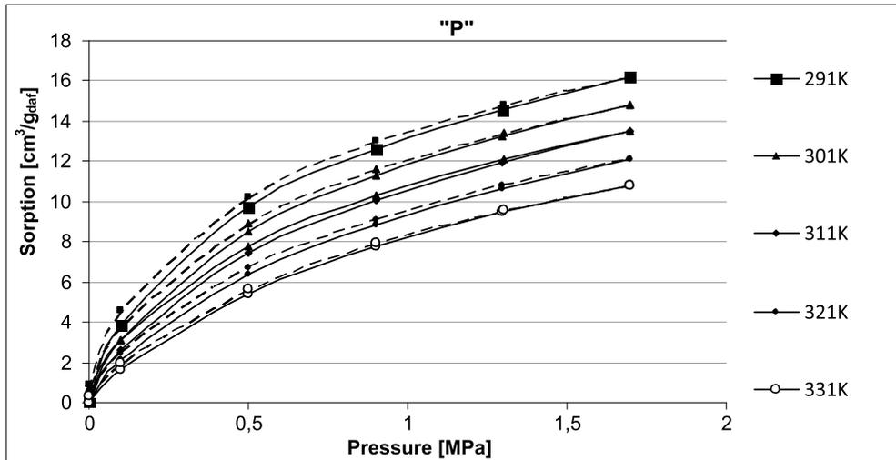
Fig. 1. Methane sorption isotherms for different temperatures
