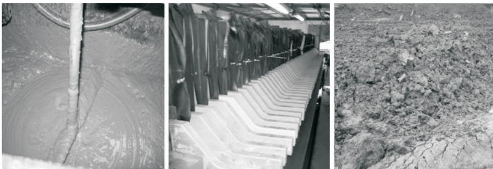
Fig. 1. Photo of used drilling mud, filtration press, and filtration cake destined for ground reclamation
