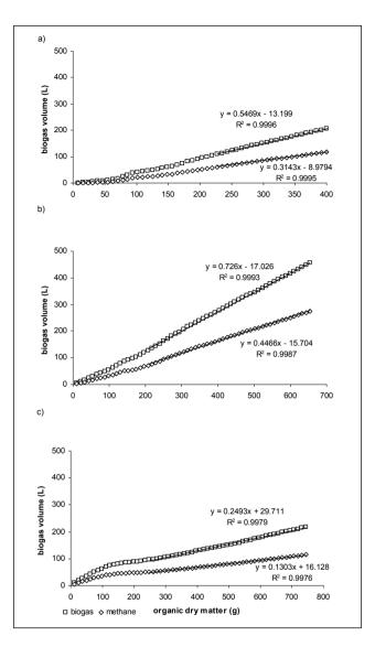
Fig. 4. Accumulated biogas and  $CH_4$  production versus added ODM during mesophilic anaerobic digestion of maize silage (run 1) and maize silage mixed with 5% (run 2) and 10% w/w (run 3) residual glycerine
