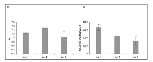
Fig. 2. Mean pH (a) and alkalinity (b) values after digestion of maize silage (run 1) and maize silage mixed with 5% (run 2) and 10% w/w (run 3) residual glycerine; (error bars represent standard deviations)
