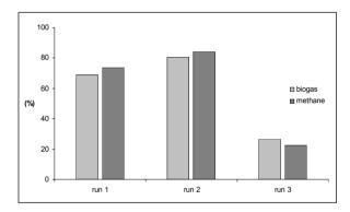
Fig. 5. Percentage of measured biogas yield  $(Y_{\text{biogas}})$  and  $\text{CH}_4$  yield  $(Y_{\text{methane}})$  in relation to theoretical biogas potential (TBP) and  $\text{CH}_4$  potential (TMP) during mesophilic anaerobic digestion of maize silage (run 1) and maize silage mixed with 5% (run 2) and 10% w/w (run 3) residual glycerine
