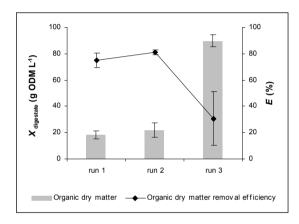
Fig. 1. Concentration of organic dry matter in the digestate (in g ODM L<sup>-1</sup>) and the efficiency of ODM removal (*E*) during the digestion of maize silage (run 1) and maize silage mixed with 5% (run 2) and 10% w/w (run 3) residual glycerine (error bars represent standard deviations)
