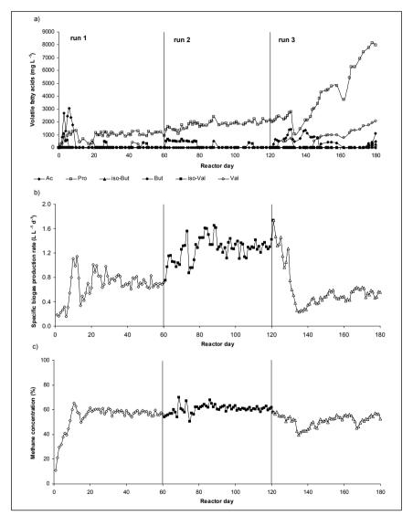
Fig. 3. Concentration of individual VFAs in the digestate (a); specific biogas production rate (b); and CH<sub>4</sub> concentration (c) during mesophilic anaerobic digestion of maize silage and maize silage mixed with 5% and 10% w/w residual glycerine (Ac – acetic acid; Pro – propionic acid; iso-But – isobutyric acid; But – butyric acid; iso-Val – isovaleric acid; Val – valeric acid)
