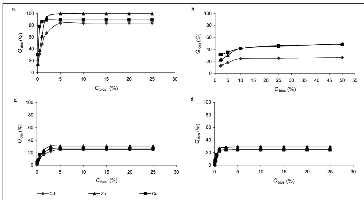
**Fig. 5.** Effectiveness of metals removal ( $Q_{des}$ ) from activated sludge immobilized in a mixture of 1.5% alginate with 0.5% PVA depending on biosurfactant concentration ( $C_{bios}$ ) using solutions of: a. saponin, b. tannic acid, c. JBR 515, and d. JBR425]
