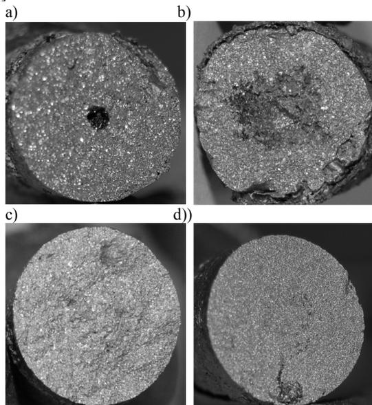
Fig. 6. Macrostructures in fractured experimental castings: FeAl -  $Al_4C_3$  – (a), FeAl - TiC – (b), FeAl - TiC with addition Mg - (c), FeAl - VC – (d)
