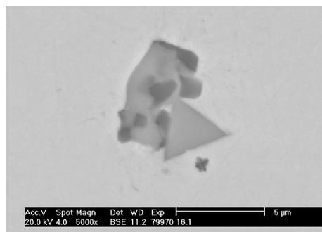
Fig. 8. Needles of aluminium nitride (5,000 x)
