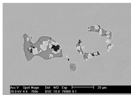
Fig. 4. Complex inclusions after deoxidation with Al+Zr (750 x)
