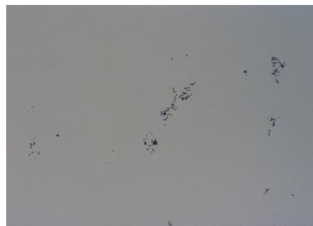
Fig. 3. Inclusions of the IV<sup>th</sup> type (100 x)
