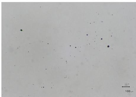
Fig. 1. Aluminium oxides with the MnS envelope (100 x)
