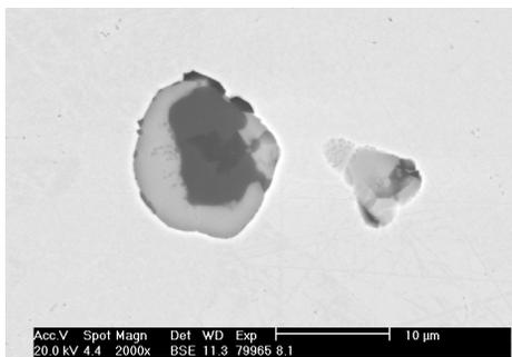
Fig. 2. Aluminium oxides with the MnS envelope (2,000 x)
