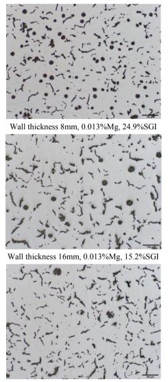
Wall thickness 40mm, 0.013%Mg, 1.5%SGI
