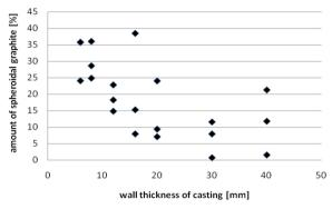
Fig. 3. Amount of spheroidal graphite depending on wall thickness of casting
