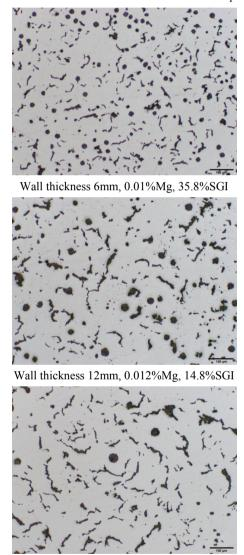
by visual analysis, in the course of which the ratio of the contents in compacted graphite and spheroidal graphite as well as graphite size and feritte and pearlite amount have been evaluated. Most customers require that the amount of spheroidal graphite does not exceed 20 %. No lamellar graphite is acceptable.
