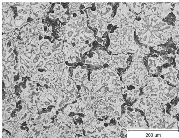
Fig. 6 Inoculated material AZ 91 the casting central part
