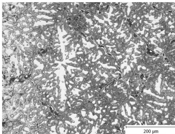
Fig. 5 Non-inoculated material AZ 91 the casting edge
