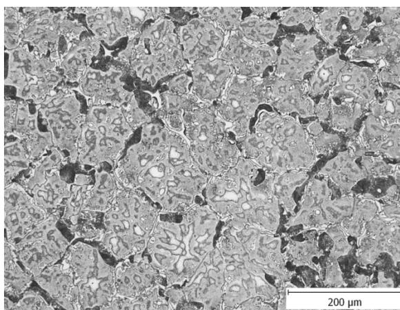
Fig. 7. Inoculated material AZ 91 the casting edge
