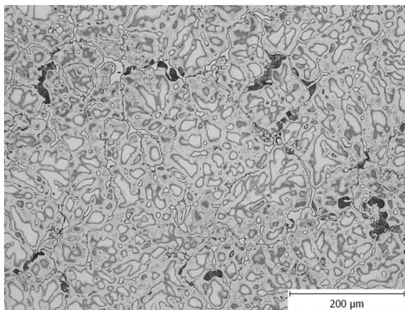
Fig. 4. Non-inoculated material AZ 91 the casting central part
