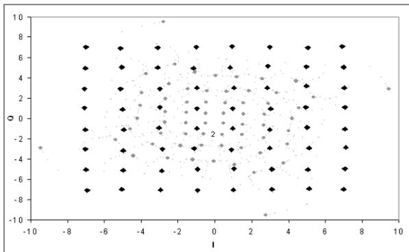
Fig. 16. Response of the HPA model with a predistorted constellation
