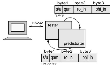
Fig. 13. Simplified diagram of Hardware testing set.
