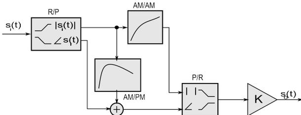
Fig. 2. Memoryless behavioral model of power amplifier.
