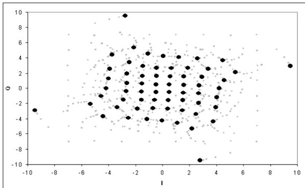
Fig. 15. Distorted 64QAM constellation obtained in 20 teaching rounds. The teaching convergence paths are marked with gray dots.
