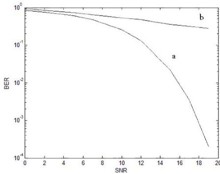
Fig. 5. Undistorted (a) and distorted (b) bit error rate for 64QAM.
