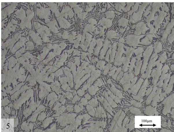
Fig. 3. AISi11 alloy structure: 1 – node; 2 – near node cross-section; 3- cross-section between the nodes; 4- cross-section of closing wall; 5 – outside surface of closing wall
