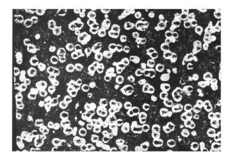
Fig.6. Cast iron of EN-GJS 500-7 grade. Pearlitic-ferritic structure P70, etched with Mi1Fe. 100x
