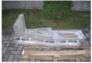
Fig. 4. Casting of the base weighing 102 kg. GJS 400-15
