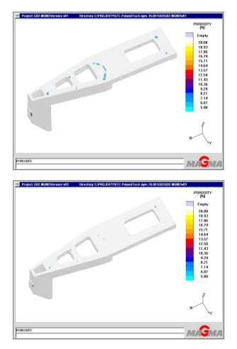
Fig. 2. The distribution of porosity above 5% for compositions S1 and S3 given in Table 1
