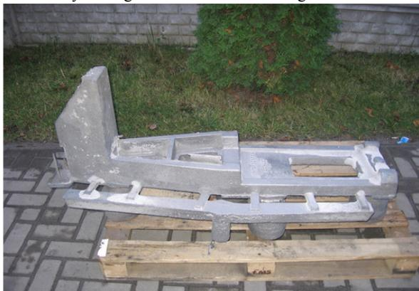
Fig. 4. Casting of the base weighing 102 kg. GJS 400-15
