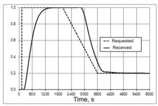
Fig. 3. Diagram changes of scaled temperature in the chamber of resistance furnace in the system with optimally selected parameters for PID controller
