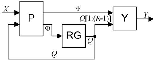
Fig. 3. Structure of logic circuit of PY<sub>J</sub> FSM.
