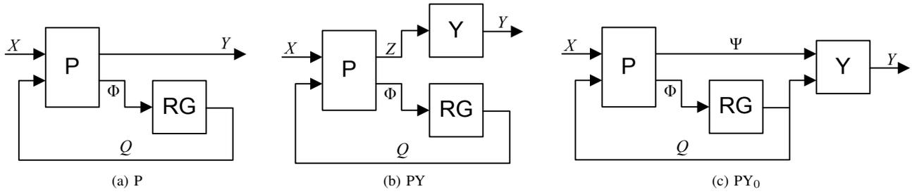
Fig. 2. Structures of logic circuit of FSM.
