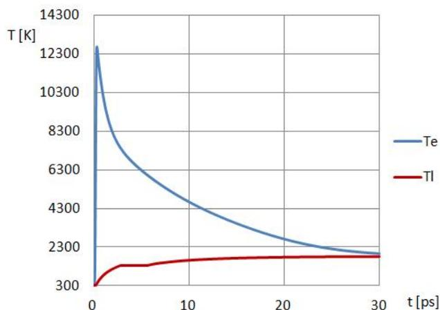
Fig. 2. Electrons and lattice temperature profiles on the irradiated surface –  $I_0 = 12000$  J/m<sup>2</sup>
