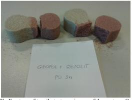
Fig. 5b. Fracture of tensile test specimens of the system: Geopol + Rezolit (after 3h)
