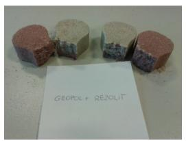
Fig. 5c. Fracture of tensile test specimens - after 24h – of the system: Geopol + Rezolit (The fracture of the tensile test specimen of the system: Geopol+Rezolit after 3h - occurs in the sand with the Rezolit
