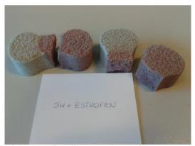
Fig. 5f. Fracture of tensile test specimens of the system: waterglass + Estrofen, after 24h
