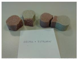
Fig. 5d. Fracture of tensile test specimens – after 24h – for the system: Geopol + Estrofen (The fracture of the tensile test specimen of the system:
