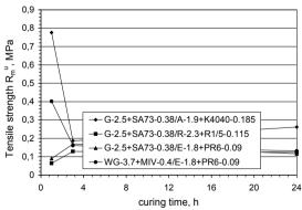
Fig. 4. Tensile strength of two-layer test specimens. Notations: G – Geopol, E – Estrofen, A – Avenol, R – Rezolit, WG – water-glass
