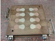
Fig. 3. Two-layer tensile test specimen for measuring the tensile strength after compaction
