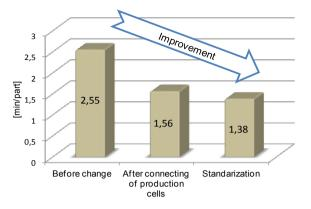
Fig. 6. Labour intensity of cast finishing operations
