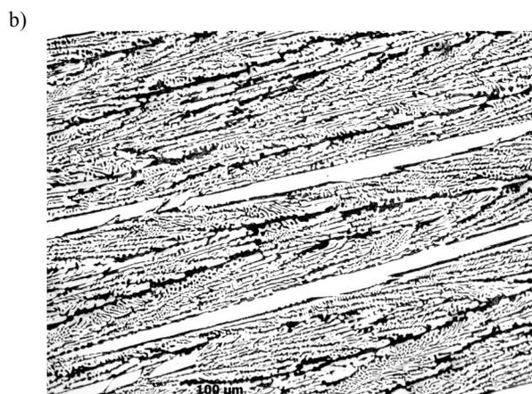
Fig. 7. Microstructure of a) eutectic, b) hypereutectic structure areas - samples after solidifying was frozen (immediately taken off the cooler),  $v=83.3 \mu\text{m/s}$ ,  $G= 33.5 \text{ K/mm}$
