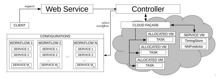
Fig. 1. The overall configuration of the developed system
