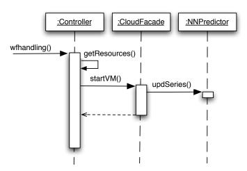
Fig. 6. Sequence diagram showing interactions with a cloud and the resource usage predictor
