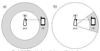
Fig. 3. Cell-ID positioning method a) omnidirectional antennas, b) sectorized antennas
