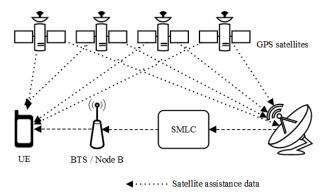
Fig. 5. A-GPS positioning method
