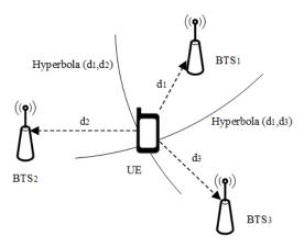
Fig. 1. TDoA positioning method
