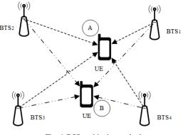
Fig. 6. RSS positioning method
