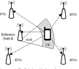
Fig. 2. AoA positioning method
