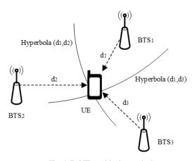
Fig. 4. E-OTD positioning method
