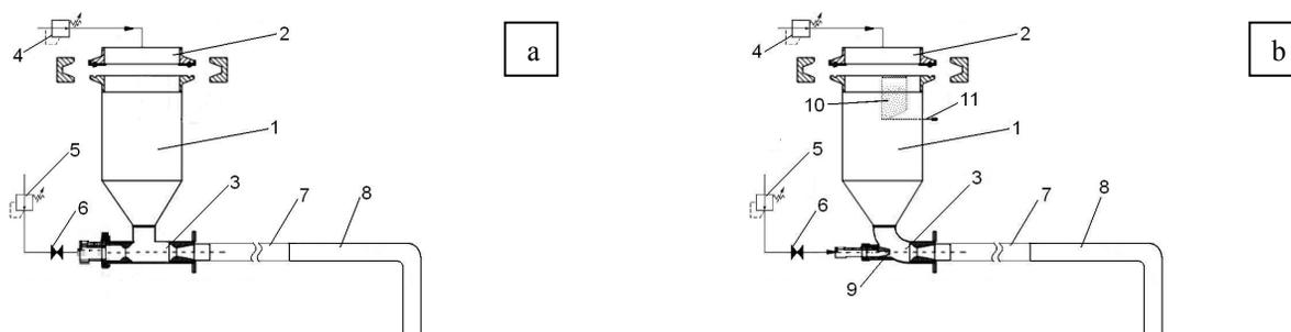
Fig. 1. The scheme of a feeder for the injection of inoculant: a) the initial stand, b) the stand after modification; 1 – pressure vessel; 2 – pressure clamp; 3 – dosing chamber; 4 – pressure regulator; 5 – carrier gas pressure regulator; 6 – electrovalve; 7 – conveying pipe; 8 – the lance injecting master alloy into metal bath; 9 – regulation nozzle; 10 – inoculant storage bin; 11 – shutter
