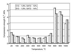
Fig. 7. Dependence of the final compression strength on the heating temperature of the moulding sand with the GEOPOL and SA 72 hardener (G - Geopol)
