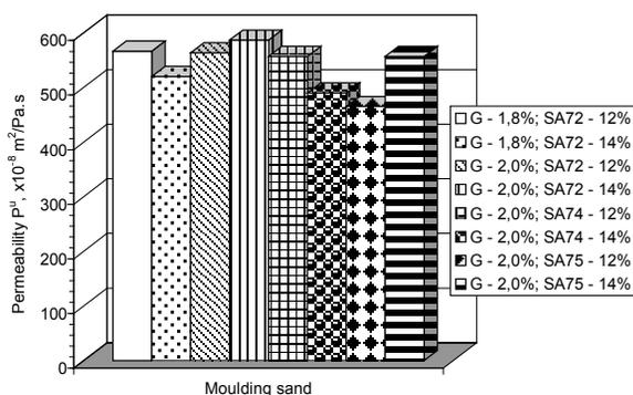
Fig. 5. Dependence of the permeability on the hardening time of the moulding sand with the GEOPOL and SA 72, SA 74 and SA 75 hardeners (G - Geopol)
