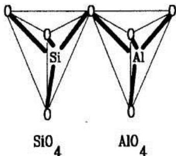
Fig. 1. Structure of a geopolymer. Geopolymers belong to alkaline aluminosilicates
